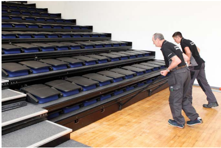
Manual operation via removable pull handles.
