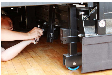
Bolted construction is continuously adjustable throughout system life to keep system running smoothly and reduce risk of wear and / or jamming.
