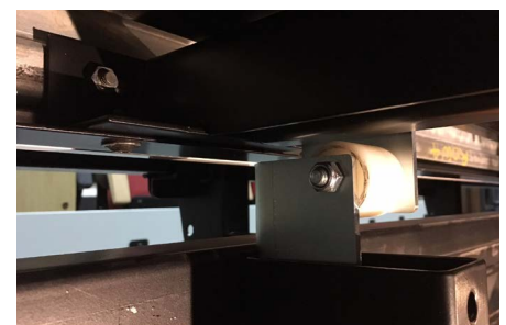
Designed to eliminate metal-to-metal contact to reduce wear, warping and noise.
